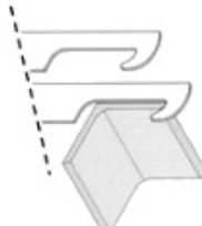
Type L For angle iron (in different sizes)
